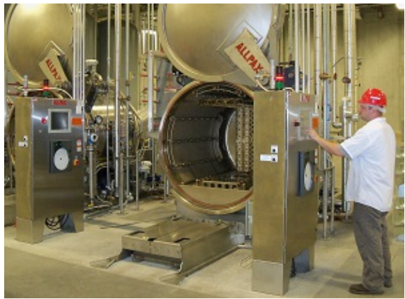
Rapid back-and-forth motion of the retort basket speeds processing in the Shaka system, which is gaining renewed interest thanks to the expiration of licensing fees. Photo: Allpax Products Inc.
